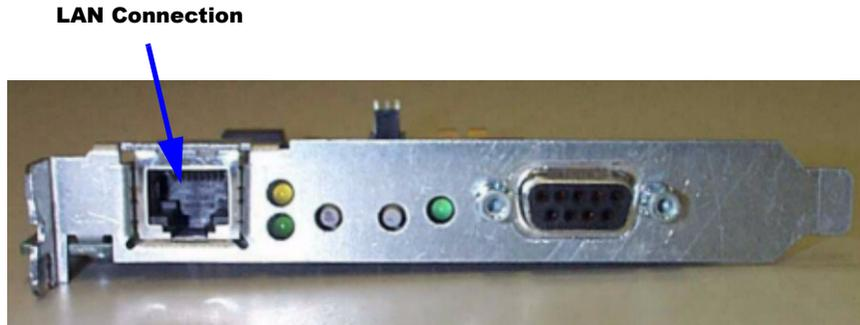
**Step 2.** Observe the LEDs on the SWC card rear bulkhead connector.
